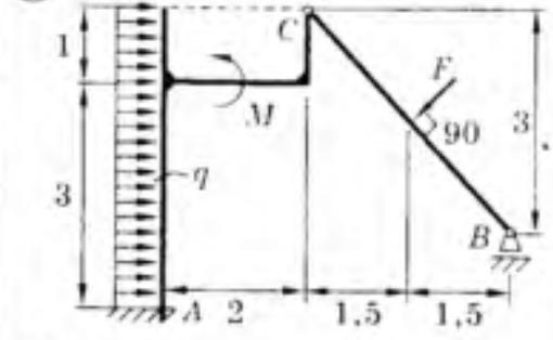
$M = 11 \text{ кН}\cdot\text{м}; q = 4 \text{ кН}/\text{м}; F = 13 \text{ кН}$
