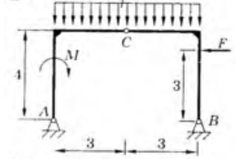
$M = 60 \text{ кН}\cdot\text{м}; q = 20 \text{ кН}/\text{м}; F = 30 \text{ кН}$
