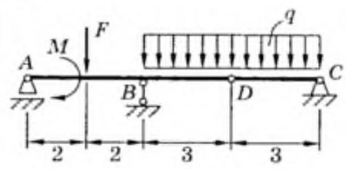
$M = 65 \text{ кН}\cdot\text{м}; q = 20 \text{ кН}/\text{м}; F = 30 \text{ кН}$
