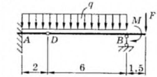
$M = 42 \text{ кН}\cdot\text{м}; q = 15 \text{ кН}/\text{м}; F = 20 \text{ кН}$
