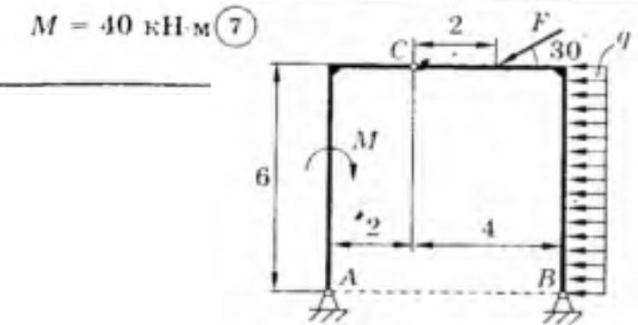
$M = 30 \text{ кН}\cdot\text{м}; q = 10 \text{ кН}/\text{м}; F = 15 \text{ кН}$
