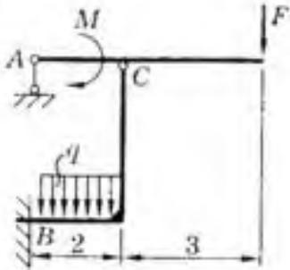
$M = 40 \text{ кН}\cdot\text{м}; q = 20 \text{ кН/м}; F = 20 \text{ кН}$
