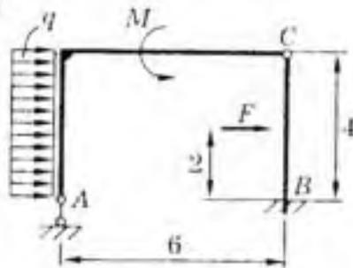
$M = 40 \text{ кН}\cdot\text{м}; q = 10 \text{ кН/м}; F = 30 \text{ кН}$
